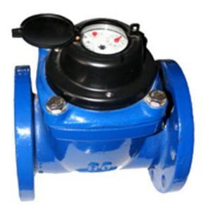
HWE Woltman Type Bulk Flow Meters are best suited for the measurement of large quantities of water for private and industrial uses. These meters are designed for maximum durability, accuracy of registration and trouble free service with little loss of head. They conform to ISO4064 B class.
